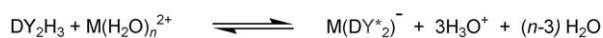
Scheme 2. Binding of M II ions to the scaffolds. The asterisk designates a noncovalently participating phenolic arene.
